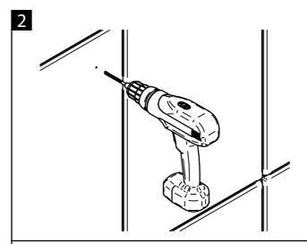
Using a 6mm drill bit, drill the marked holes and insert the wall plugs i f required.
