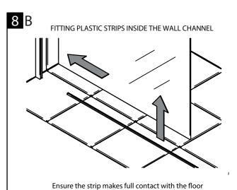
position the strip onto the bottom of the panel, flush with the front edge, then carefully push into the wall channel.
