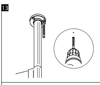
Mark the position of the holes on the ceiling, unlock and lower the inner pole, then drill the positions marked.
