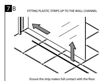
Position the strip onto the bottom of the panel, flush with the front edge, then carefully push the panel into the wall channel.
