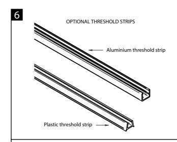
If using the threshold strip, there are 2 types available and 2 fitting options: fitting up to the wall channel (stage 7), fitting inside wall channel (stage 8).
