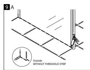
Apply silicone sealant along the bottom of the panel and wall channel and 50mm up the wall channel.
