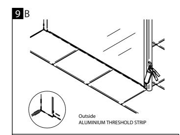
Apply silicone sealant along the bottom of the threshold strip and wall channel, 50mm up them wall channel and up the joint between the wall channel and threshold strip.
