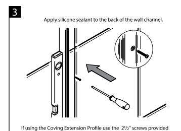
Place the washers over the  $1^{1}/_{2}$ " screws and screw the wall channel into position, ensuring it remains vertical.
