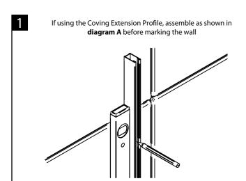
Place the wall channel in desired location and mark position of the four holes onto the wall.
