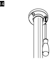
Raise the inner pole, lock in position and screw the ceiling bracket in place.
