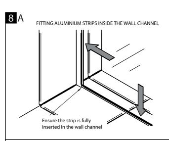
Position the strip inside the wall channel. At the same time, angle the panel and carefully push into the wall channel and threshold strip.
