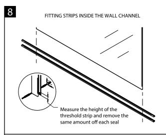
Remove the panel. Carefully trim your chosen threshold strip down to the same width as the panel.
