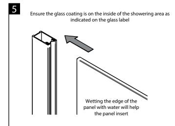
Place the glass panel into the wall channel (correct way around) and temporarily attach the floor to ceiling pole.
