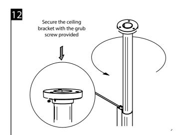
Fit the ceiling bracket to the inner pole. Then extend the pole to required height and rotate it until it locks in the position.
