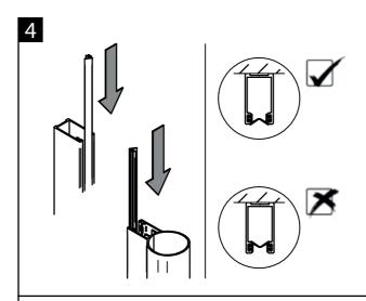
Slide both seals down into the channel and cut off any excess. **Note the orientation of the soft flippers.**
