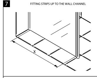
Carefully measure the distance between the wall channel and the supreme outer pole (X), then trim your chosen threshold strip to length (X). Remove the panel.
