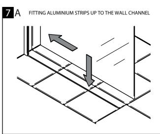
Position the strip up against the wall channel. At the same time, angle the panel and carefully push into the wall channel and threshold strip.
