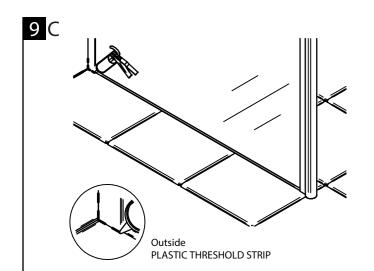
Apply silicone sealant along the bottom of the wall channel and 50mm up the wall channel.
