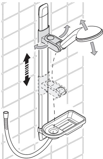
2. Slide the Clamp Bracket up and down the Slide Rail until the Showerhead is positioned to your preference.
