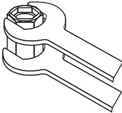
Hold a spanner or other suitable grips across flats of the metal connector. Unscrew filter using another spanner as shown. Clean or replace filter as necessary. Refit filter making sure it is screwed fully home. **Do not overtighten.**
