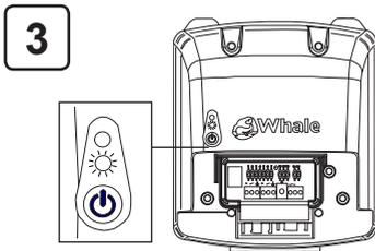
Press the start button and hold for 7 seconds, the light will flash **green** and **red** indicating that it has entered pairing mode.
