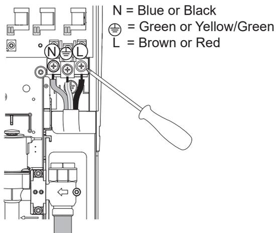
Feed the electrical cable into the case. Firmly connect the conductors. **DO NOT** exert strain on the terminal block.
