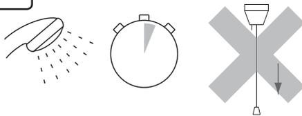
Appliance will purge water from heater tank for a few seconds.
