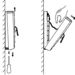
Remove cover screw, cover and splash guard. Disconnect ribbon cable from cover
