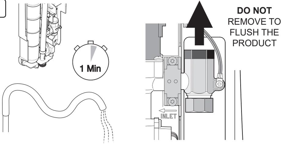
**DO NOT** flush through the product by removing the inlet filter. Debris may damage the product and invalidate the guarantee.
