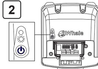
Turn on the power to the pump. The light will flash **red** every 4 seconds indicating that it is not paired.
