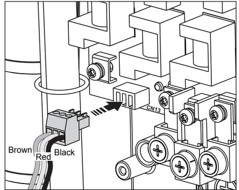
1. Remove the male connector from the relay PCB (CN13).
