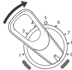
Turn the temperature control to the full hot position and continue to run the shower for at least 1 minute.
