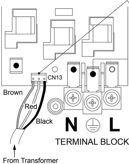
3 wires signal cable connection to relay board
