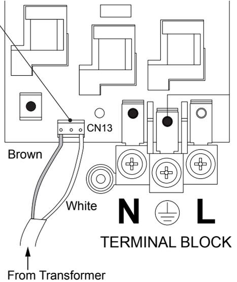
2 wires signal cable connection to relay board
