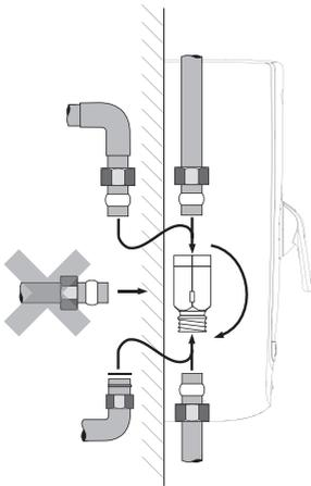
Turn the inlet connector to suit supply pipe. **Do not** trap the green wire.
