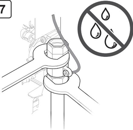
Connect supply pipe, then turn the water supply on and check the shower unit for leaks. **DO NOT** overtighten.
