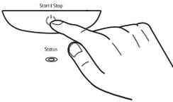
Start the shower to test for water flow. The shower will beep once (3 times when set in BEAB mode) and the white start/stop light and orange status light (green in BEAB Mode) will pulse. Wait until the lights go solid and the shower will beep again.
