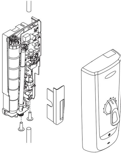
Remove the cover, the service tunnel and the bungs. Determine the cable and pipe supply either top or bottom or rear connection.
