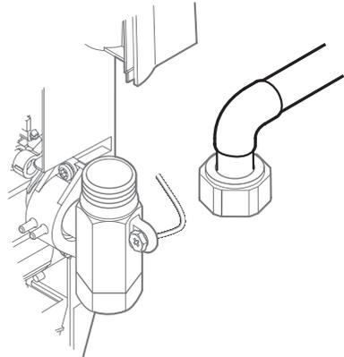
Complete any soldering required away from the appliance.
