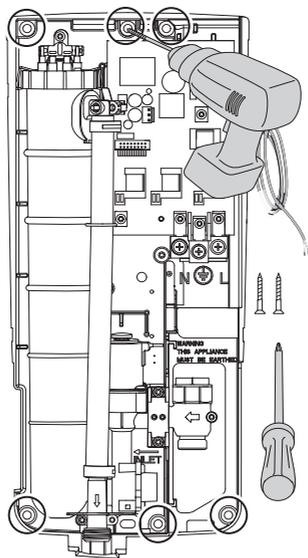
Drill the fixing holes through the plastic case in the designated areas as required.
