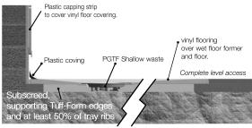
**Step 1.** Position the TuffForm over the desired location for the shower. Formers are trimmable and can be cut to down to minimum 150mm to the waste area. Ensure the cut edges are straight and put towards the wall mounted side. If necessary cut to the correct size with a suitable circular saw or a fine toothed blade. Mark around the edge of the shower former.
