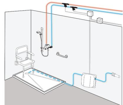
The Phlexiflow High capacity pump is the ideal solution for power showers with an output between 12 - 20 litres per minute.
