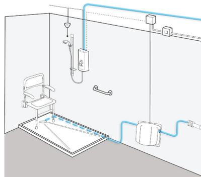
The React system allows the pump to be connected directly to the electric shower thereby eliminating the need for a flow switch.
