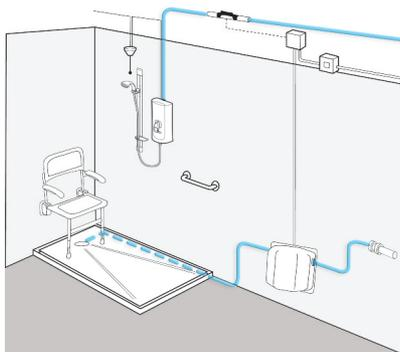
This standard kit comes with a flow switch. Factory pre-set to allow 7-9 litres of water per minute to be removed. It can be adjusted on site to cope with up to 12 litres per minute. For a mixer valve, 2 flow switches are required.
