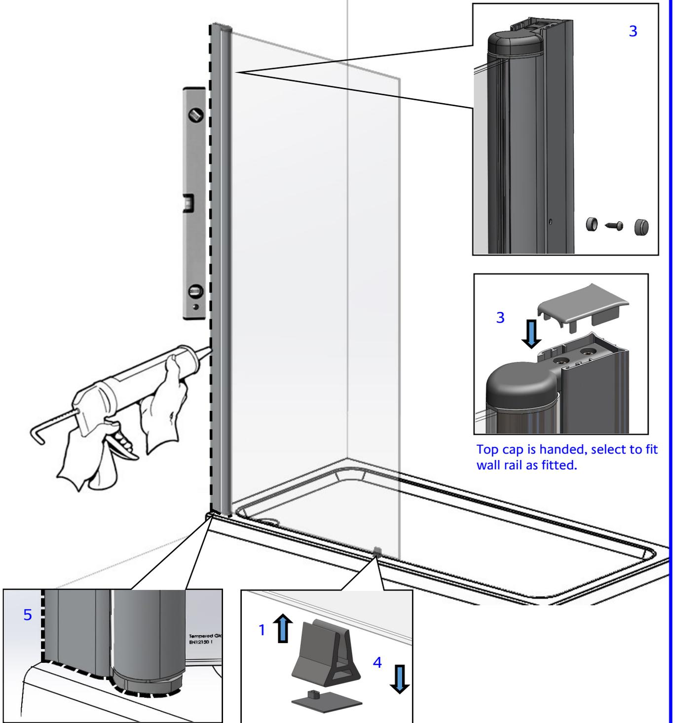
Top cap is handed, select to fit wall rail as fitted.
