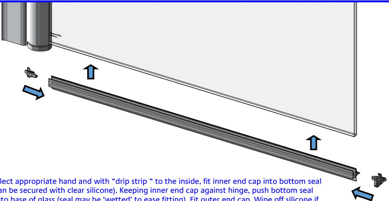
Select appropriate hand and with “drip strip “ to the inside, fit inner end cap into bottom seal (can be secured with clear silicone). Keeping inner end cap against hinge, push bottom seal onto base of glass (seal may be ‘wetted’ to ease fitting). Fit outer end cap. Wipe off silicone if this has been used with a damp cloth or alcohol wipe.
