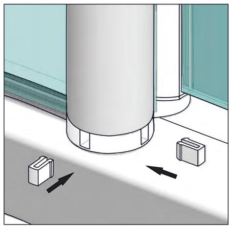
Apply clear silicone to holes & press fillers into bottom bracket. Wipe off excess sealant.
