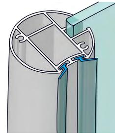
Fit hinge seals into grooves in door post
