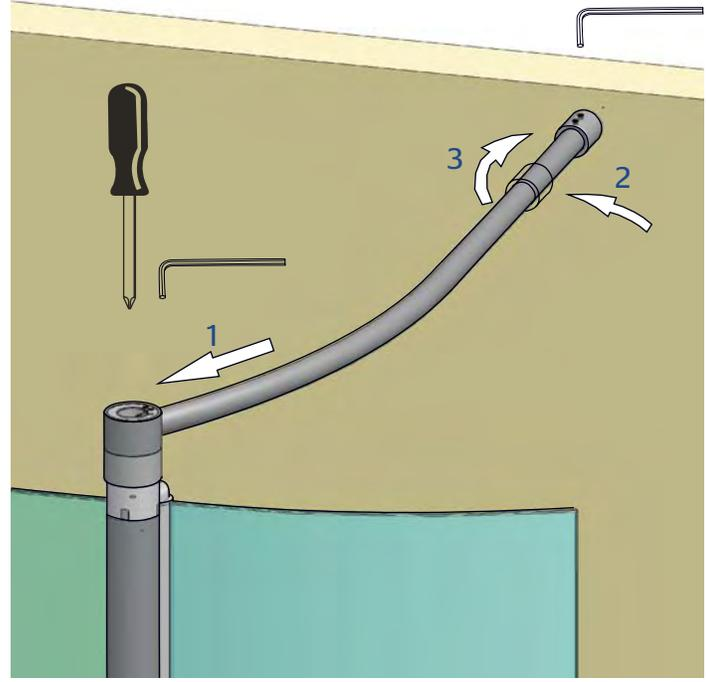
Fit Finial onto top hinge bracket using M6 x 35 C/Sunk screw.
