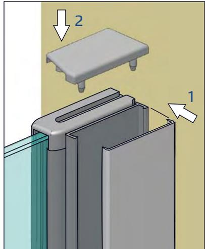
1. Align top of cover section with top of wall rail & working from top to bottom, press in over entire length.
