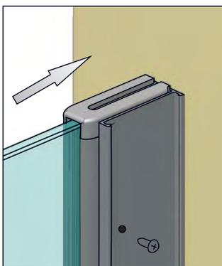
With main panel in desired position & plumb in wall profile, from inside, using wall rail holes as a guide, drill (dia 3mm) & screw main panel to wall rail (3x 3,5x10 pan head screws)
