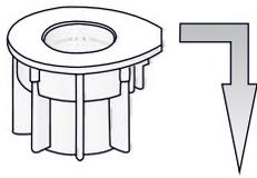
Press fit hinge bearings to door rail ends. Apply smear of silicone grease to inside dia' of plastic bearing
