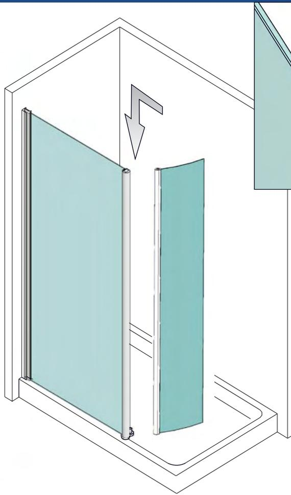
Carefully lift door onto bottom hinge & whilst supporting top of door, fit top hinge bracket & tighten (2x) 4x25 C/Sunk screws.
