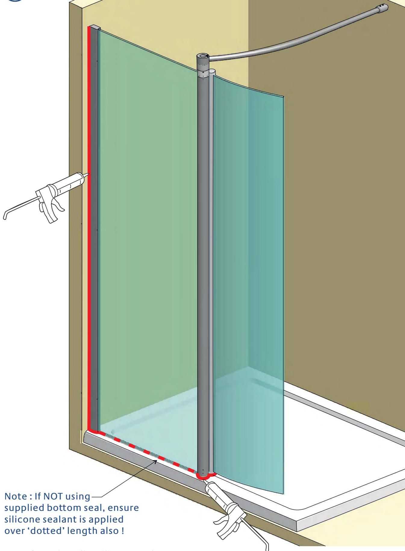
Note : If NOT using supplied bottom seal, ensure silicone sealant is applied over 'dotted' length also !
