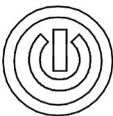
Touch sensitive **⏻** key switches the unit between on and standby modes, press and hold for 1.5 seconds to activate.
